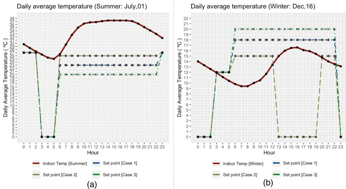
**Figure 10.** Indoor temperature in summer and winter and the setpoint for each case: (a) displays the indoor temperature for 16 December and the setpoints for each case, and (b) displays the indoor temperature for 1 July and the setpoints for each case.
