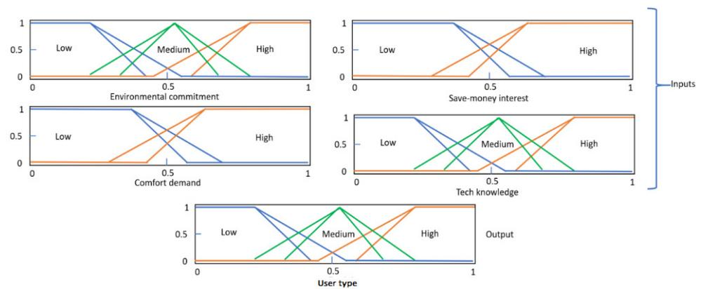
**Figure 4.** Fuzzy logic type II membership functions.
