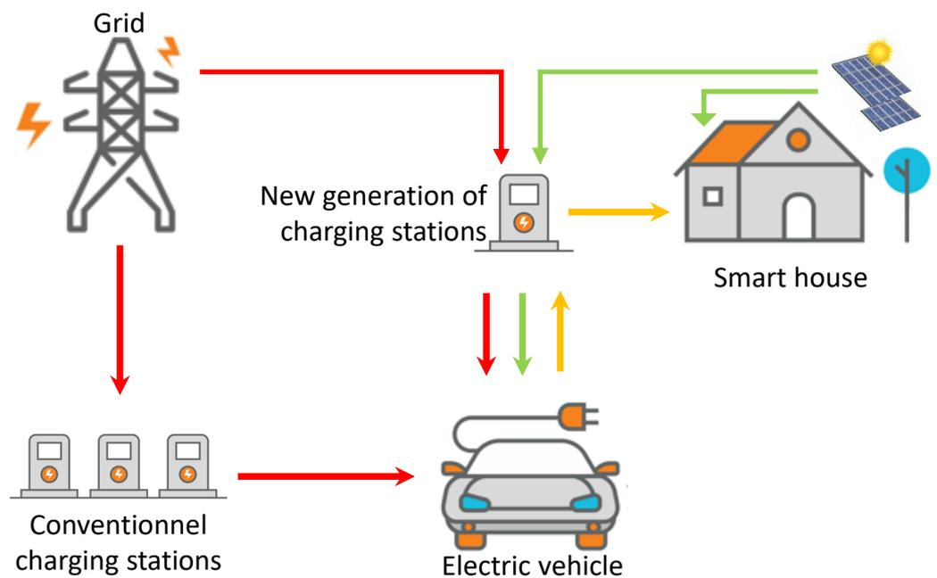
**Figure 6.** Vehicle to Grid concept.
