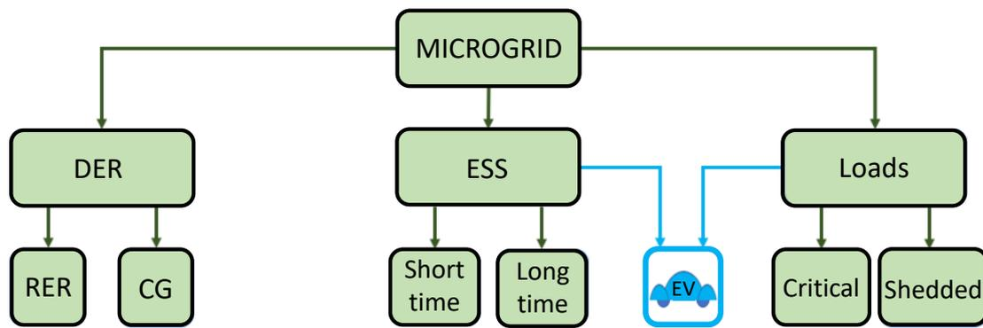
Figure 3. Microgrid components.
