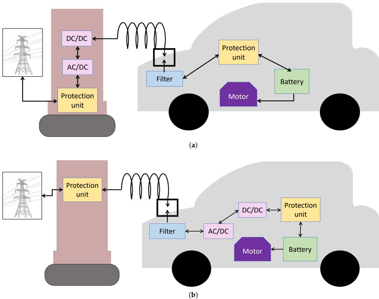
**Figure 8.** Schematic diagram of EV charging infrastructure. (a) AC charging stations. (b) DC charging stations.
