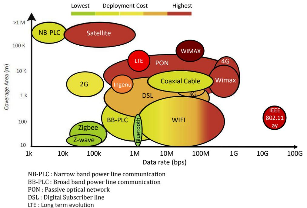
**Figure 5.** Communication technologies comparison in terms of coverage area and data rate for MGs data exchange [22].
