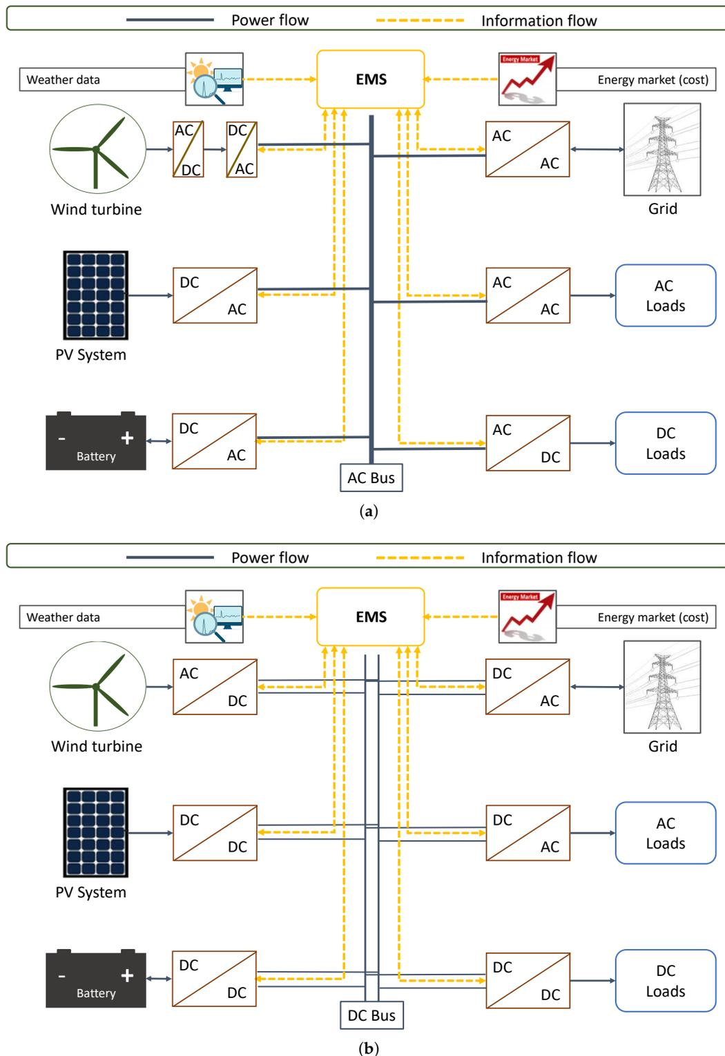
**Figure 10.** Renewable resources-based AC and DC microgrids architecture. (a) AC microgrid topology. (b) DC microgrid topology.
