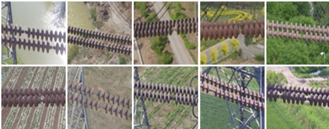
**Figure 7.** The samples of simulated insulator fault.
