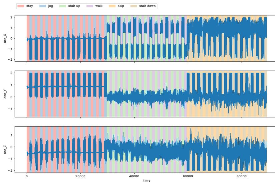
**Figure 9.** Human action recognition data for Person06023. Each row represents accelerations for  $x$ -,  $y$ -, and  $z$ -axes, respectively.
