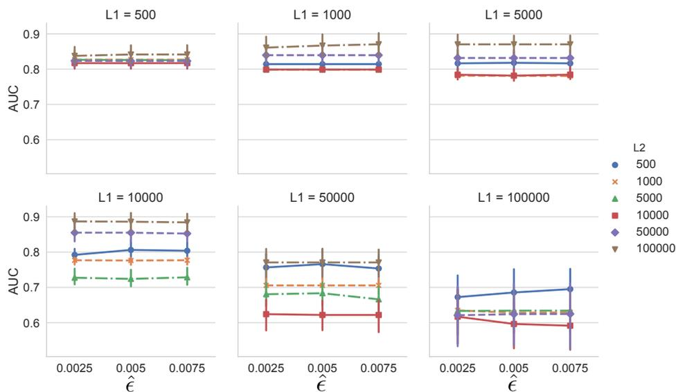
Figure 7. Dependency of AUC on threshold controlling parameter  $\hat{\epsilon}$  of SEED [13] on Synthetic Dataset 1.
