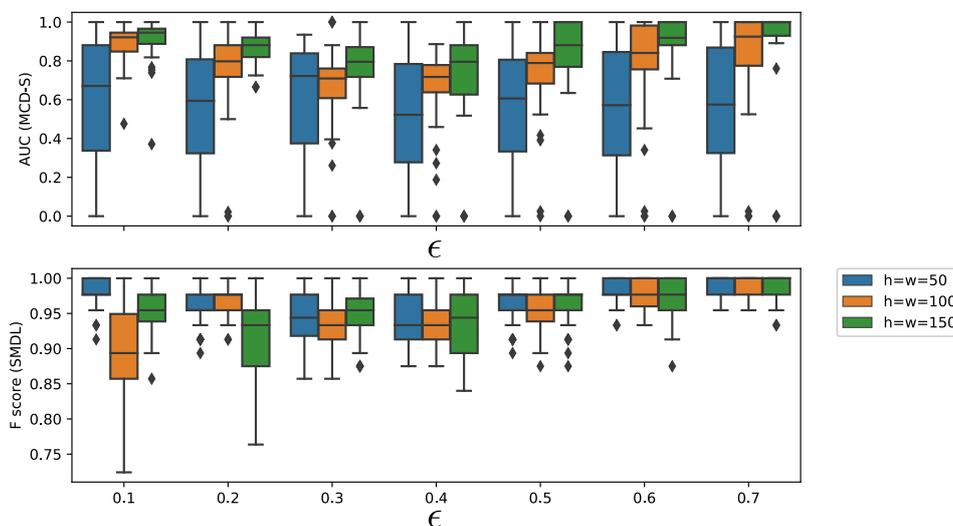
**Figure 8.** Dependency of AUC on threshold parameter  $\epsilon$  for SMDL [8] and window size  $h$  of MCD-S on Synthetic Dataset 2.
