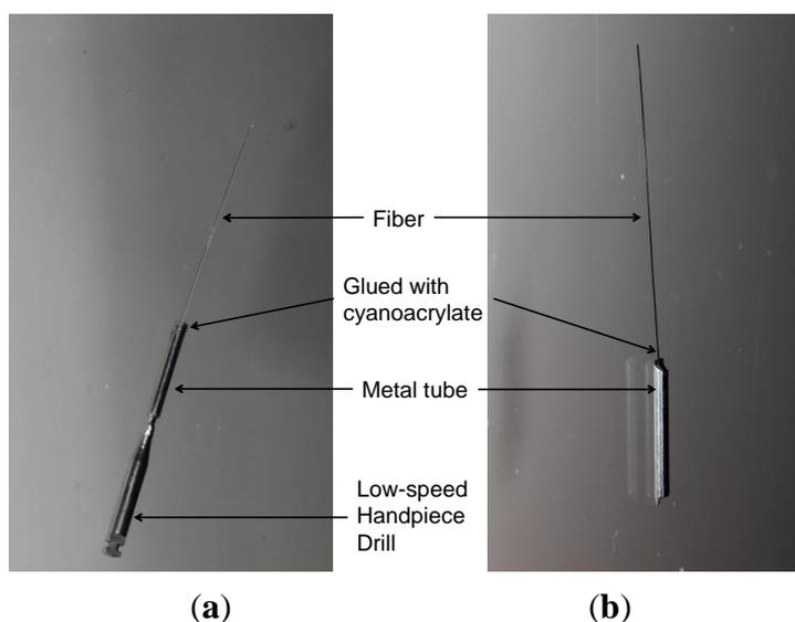
**Figure 1.** Custom-made fiber files used in this study for the low-speed hand-piece (a) and for the reciprocating EVA hand-piece (b). Note: An adaptor was used to connect the low-speed hand-piece to the metal tube.
