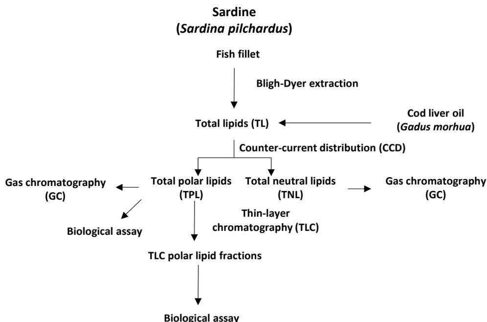
**Figure 1.** Schematic diagram of the experimental procedure that was followed.
