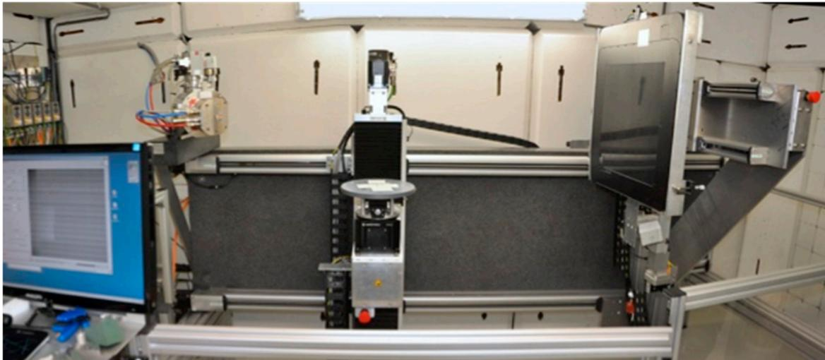
**Figure 17.** A micro-computed tomography ( $\mu$ CT) system in use at Ghent University [285].
