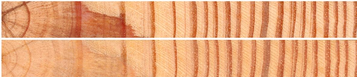
**Figure 1.** Loblolly pine radial strip before (**top**) and after (**bottom**) extraction.
