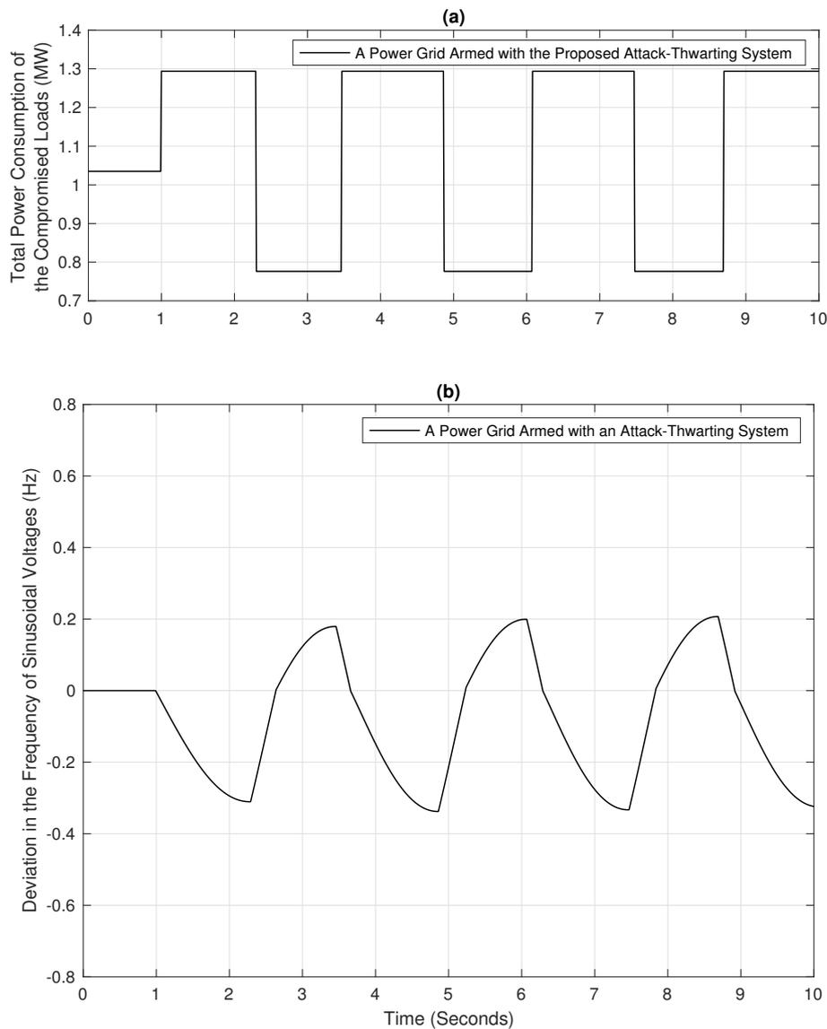
**Figure 4.** The impact of a Load Altering Attack on a power grid armed with the proposed attack-thwarting system: (a) Total power consumption of the compromised loads (b) The deviation in frequency of sinusoidal voltages in the power grid.
