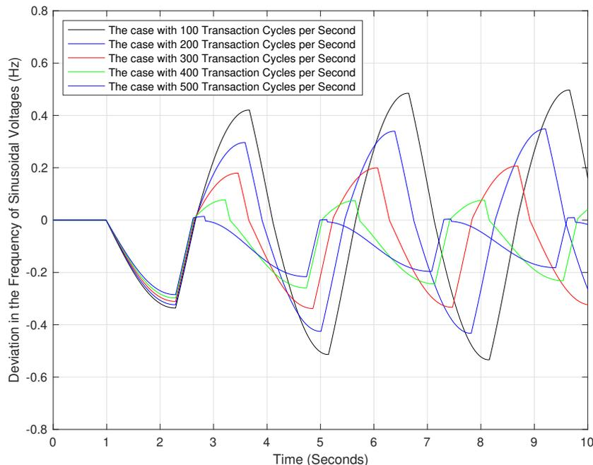
**Figure 5.** The impact of the rate of power exchanges between the power grid operator and the flexible loads, on the frequency of sinusoidal voltages.
