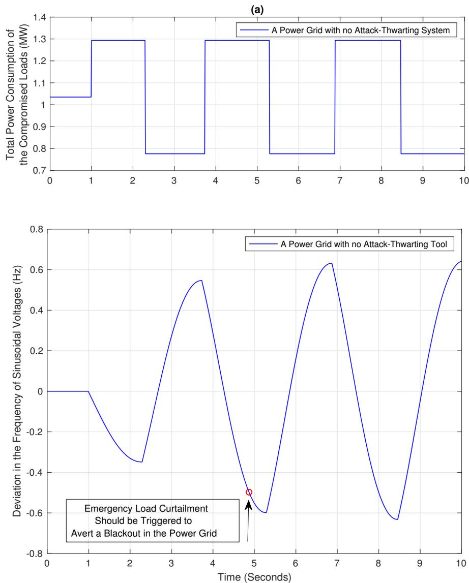
**Figure 3.** The impact of a Load Altering Attack on a power grid with no attack-thwarting system (a) Total power consumption of the compromised loads (b) The deviation in frequency of sinusoidal voltages in the power grid.
