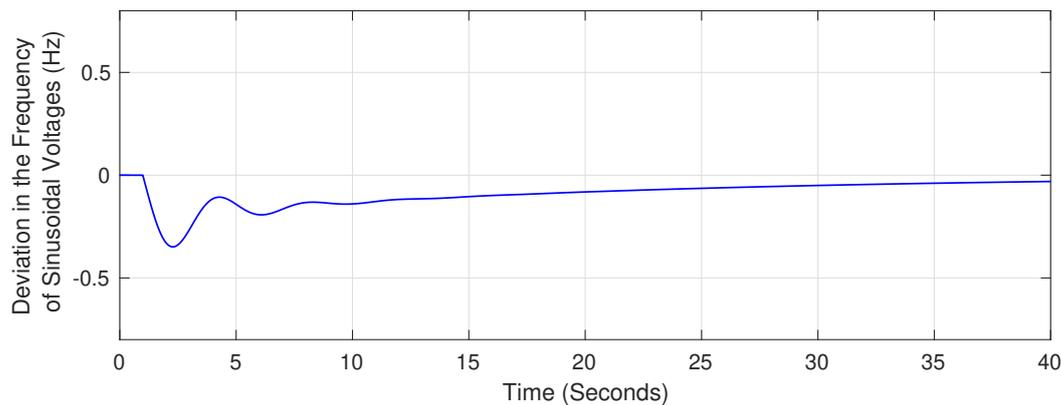
**Figure 2.** The deviation in frequency of sinusoidal voltages in a power grid, succeeding an increase in the power consumption of the grid and the corresponding response of the automatic generation control mechanism.
