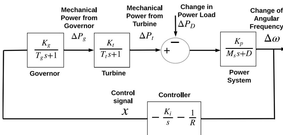
Figure 1. The representation of automatic generation control in complex frequency domain [36,37].
