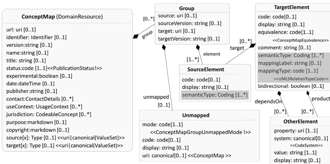
**Figure 7.** Profiled FHIR ConceptMap as a UML class diagram with designed FHIR extensions (Figure 6) as attributes (highlighted).
