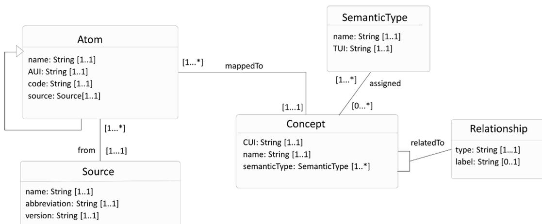
**Figure 3.** UML class diagram representing UMLS knowledge structure where the Concept class represents the UMLS concept, Atom class represents atoms in UMLS, and other classes support the Concept class.
