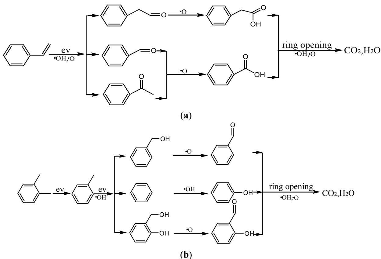
**Scheme 1.** (a) Proposed reaction pathways for the abatement of styrene in gas phase; (b) Proposed reaction pathways for the abatement of *o*-xylene in gas phase.
