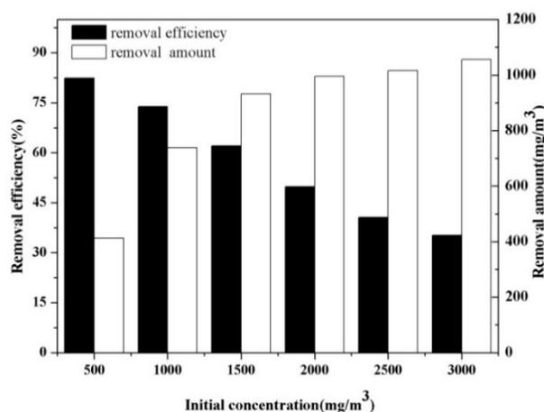
**Figure 3.** Influence of initial concentration on the decomposition of mixed VOCs.
