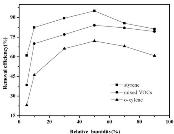
**Figure 5.** Influence of relative humidity on the decomposition of mixed VOCs.
