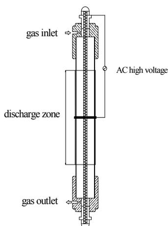
**Figure 1.** Schematic of the DBD plasma reactor.
