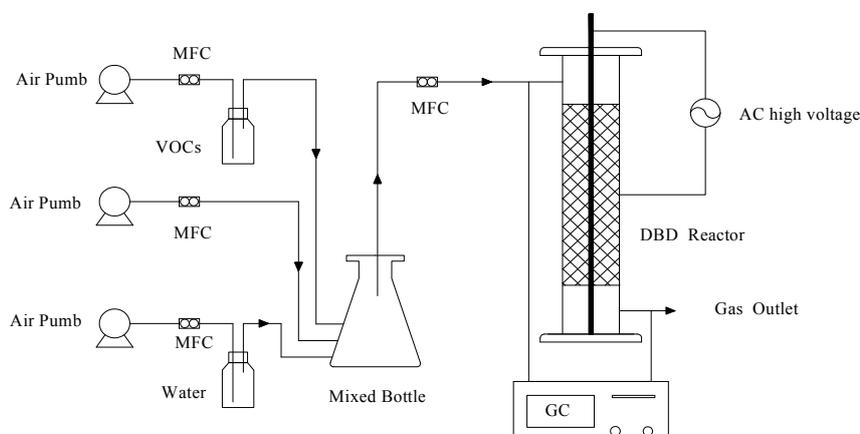
**Figure 2.** Schematic of the experimental setup.
