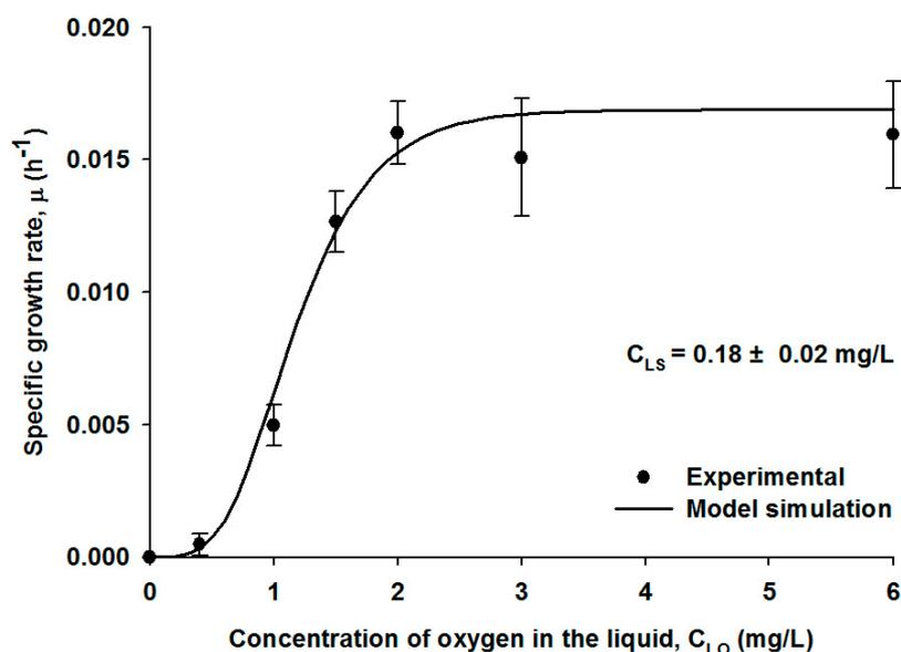
**Figure 2.** The specific growth rates of the SOB strain as a function of the oxygen concentrations in the liquid medium. The symbols show averaged experimental data with standard deviations, and the line illustrates model fitting.
