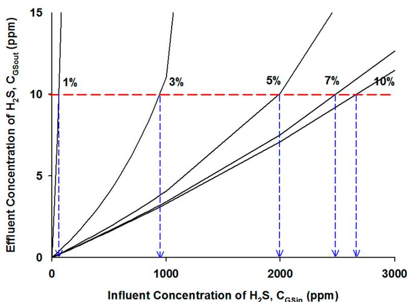
**Figure 6.** Model simulation results of the  $H_2S$  concentrations at the effluent stream at different influent  $H_2S$  concentrations and oxygen contents.
