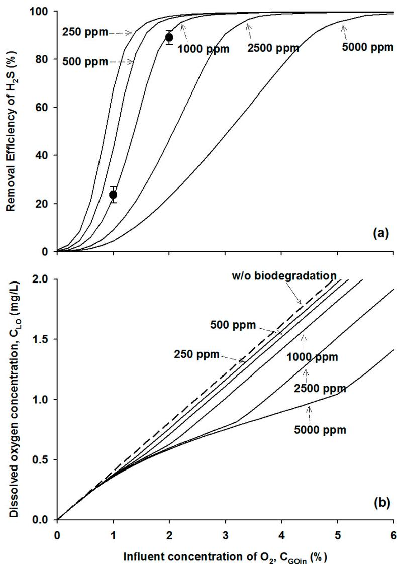
**Figure 5.** Experimental data (symbols) and model simulation results (lines) of (a) the  $\text{H}_2\text{S}$  removal efficiency and (b) dissolved oxygen concentration at different influent oxygen contents and  $\text{H}_2\text{S}$  concentrations.
