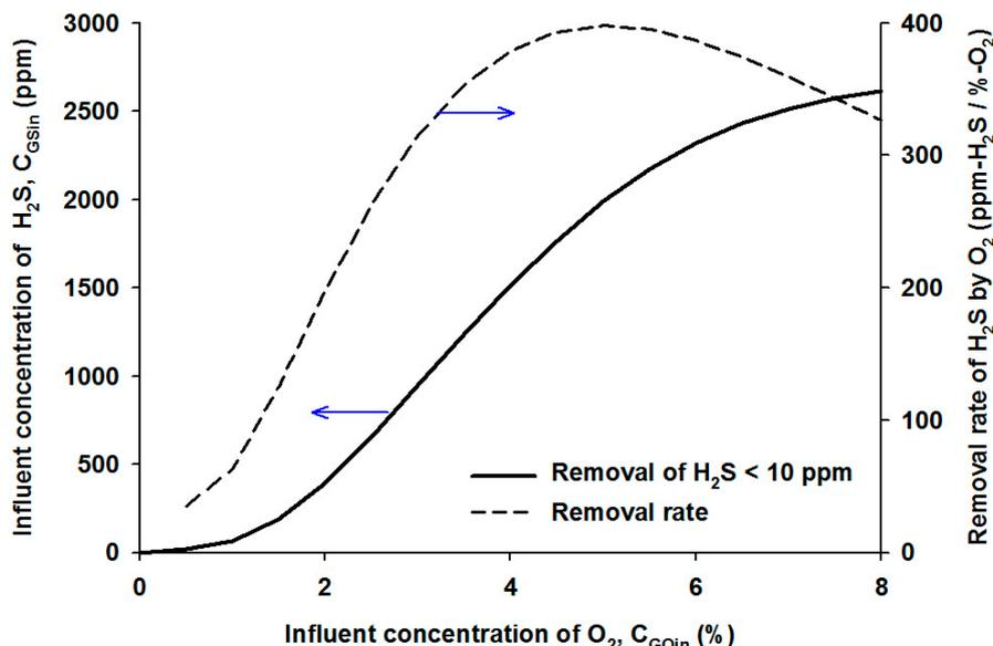
**Figure 7.** The highest inlet concentration of H<sub>2</sub>S and the specific removal rate of H<sub>2</sub>S as a function of the inlet oxygen content.
