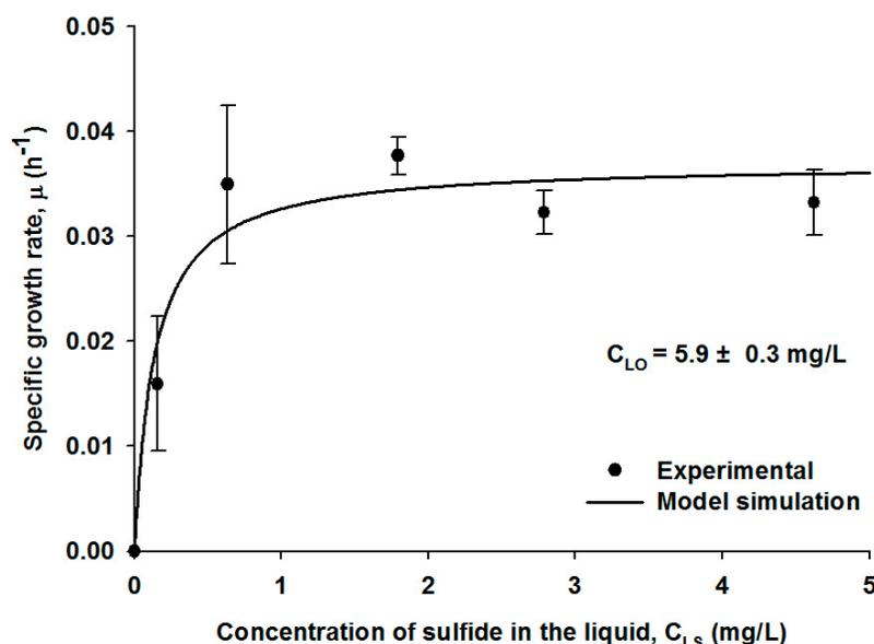
**Figure 1.** The specific growth rates of the SOB strain at different H<sub>2</sub>S concentrations in the liquid medium. The symbols show averaged experimental data with standard deviations, and the line illustrates model fitting.
