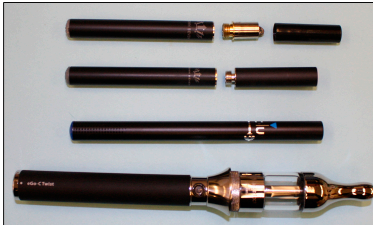
Figure S1. Layout of each generation of EC. (Top to bottom) 3- piece cartridge style, 2-piece cartomizer style, 1-piece disposable style, and tank style.
