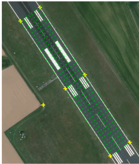
Figure 5. Basic geodetic net (yellow crosses) and recorded points for the comparative plane (green crosses).
