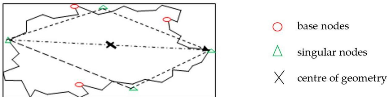
**Figure 1.** Cartographic control points of an aerial object.
