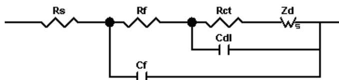
The real and imaginary values for impedance for an ideal Randle’s circuit (Figure 4) can be given as [36]:
