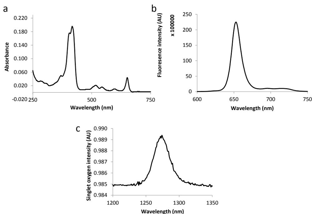
**Figure 3.** Absorption spectra (a), fluorescence emission (b) and singlet oxygen emission spectra (c) for TPC–PEG18–DKPPR in ethanol.
