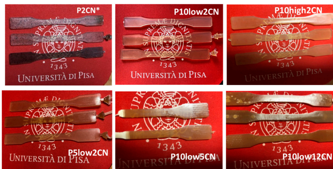
Figure 5. specimens obtained by injection moulding: comparison regarding transparency.
