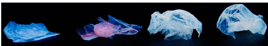
Figure 3. Digital photographs of PS-CF . From left to right: CF , P2-CF , P3-CF and P4-CF under ultraviolet light.
