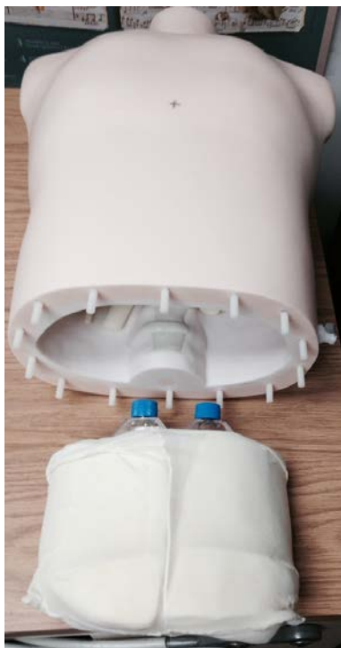
Figure 1S. 3D torso tissue-simulating phantom that was used for CT scans of hESCs in T-75 cell culture flasks placed in its abdominal cavity.
