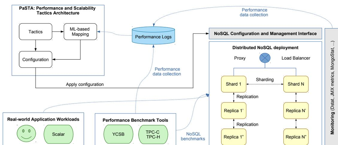
**Figure 5.** Machine learning based mapping of performance and scalability tactics through runtime configuration on NoSQL systems.
