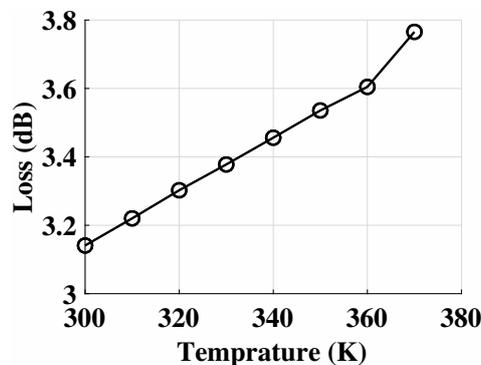
Figure 7. The effect of temperature change on propagation loss in asphalt.
