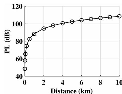
Figure 4. The path loss with change in distance.
