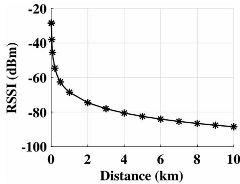
Figure 5. The received signal strength indicator with distance.
