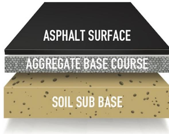
**Figure 2.** The layered structure of the underground medium.
