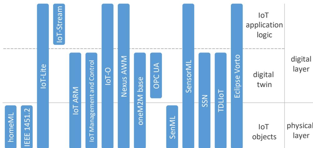
Figure 5. IoT models mapped on layers of the Internet of Things.
