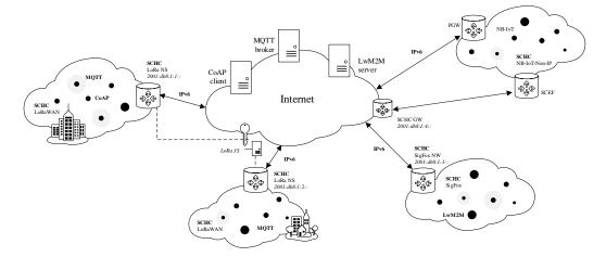
Figure 2. End-to-end secured, decentralized IPv6 Low-Power Wide-Area Network.
