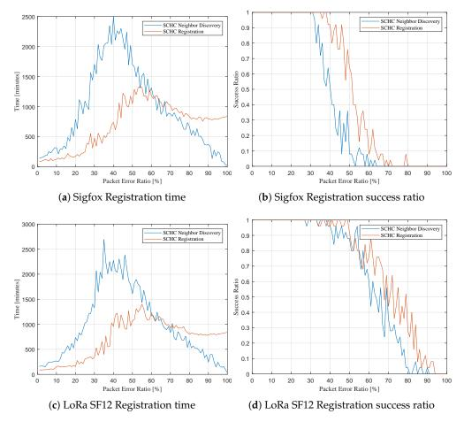
Figure 14. Registration time for different packet error ratios (PERs).
