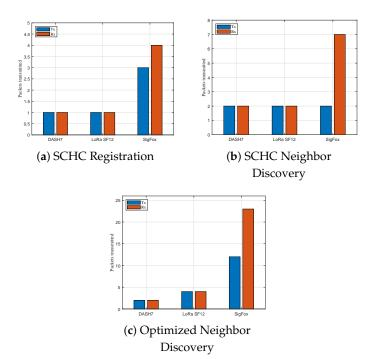
**Figure 13.** The total packet overhead for a single registration attempt using both registration mechanisms for different technologies.
