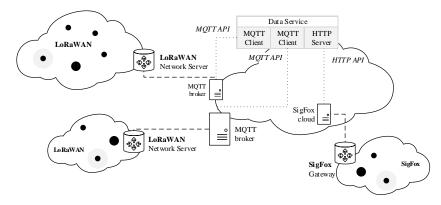
**Figure 1.** The current Low-Power Wide-Area Network landscape: centralized components deliver data to translation units.
