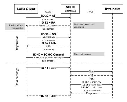
Figure 5. ICMPv6-based SCHC device and context registration.
