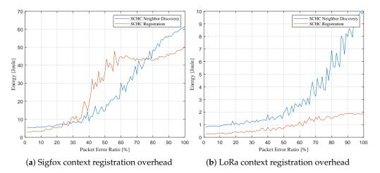
Figure 16. Energy overhead in order to configure the SCHC context for different PERs.
