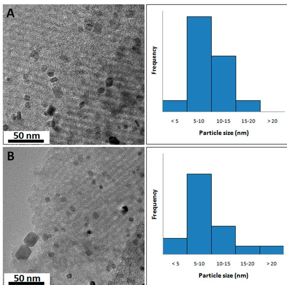
**Figure S3.** TEM picture at high magnification and TMN particle size distribution of FDU-15/CrN-850° (A) and FDU-15/VN-950° (B).
