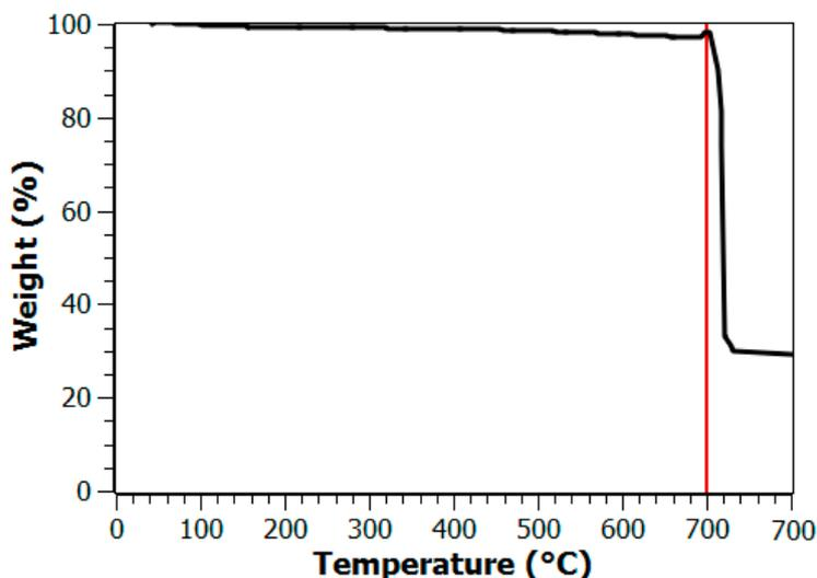
**Figure S2.** TGA curves of FDU-15/VN-950°. Heating ramp is 10 °C/min in Ar flow. At 700 °C, Ar was switched to air and temperature was maintained at 700 °C for one hour.
