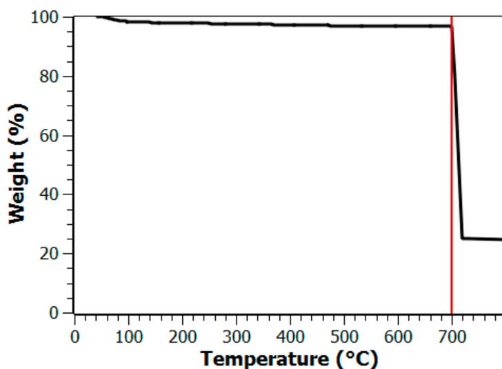
**Figure S1.** TGA curves of FDU-15/CrN-850°. Heating ramp is 10 °C/min in Ar flow. At 700 °C, Ar was switched to air and temperature was maintained at 700 °C for one hour.
