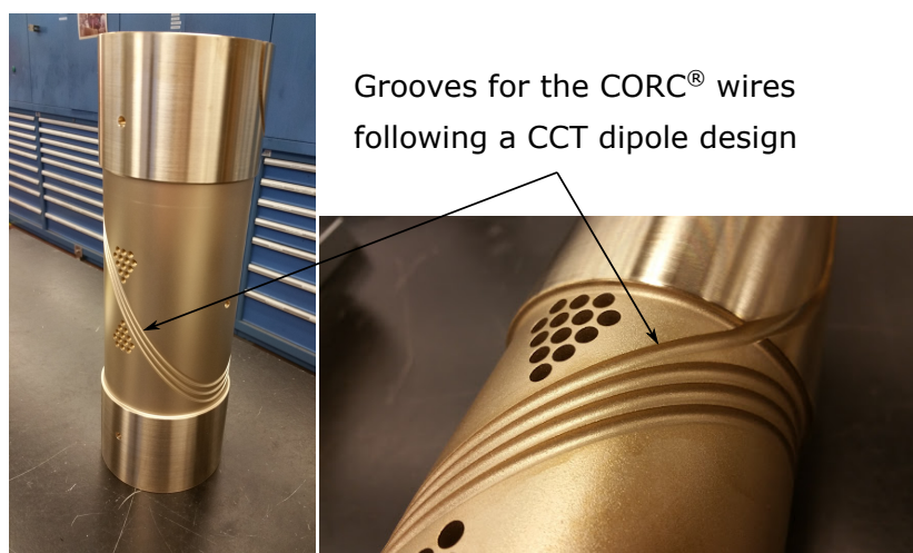
Figure 5. A three-turn aluminum bronze magnet mandrel designed by W. Ghiorso and machined by M. Maruszewski at Lawrence Berkeley National Laboratory (LBNL) for test winding of CORC ® wires.
