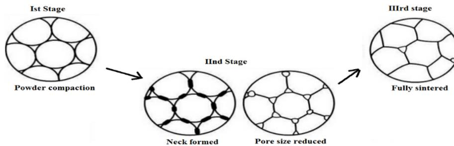
**Figure 3.** Sintering stages from powder to densification.
