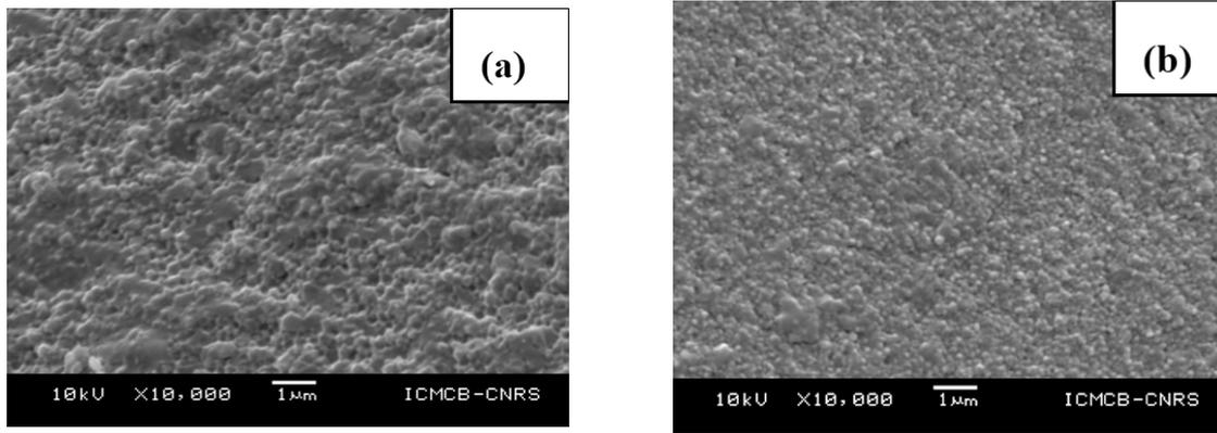
**Figure 6.** (a) Commercial HAp-SPS sintered at 900 °C, 10 min; (b) synthesized needle-shaped HAp-SPS sintered at 900 °C, 10 min.
