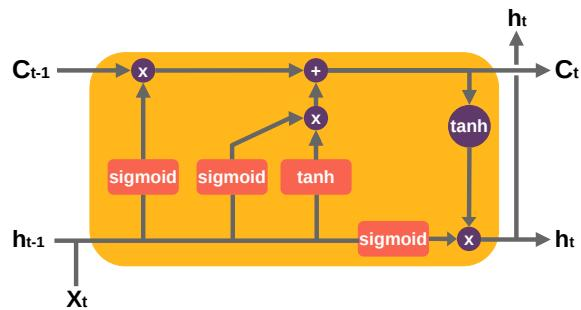
**Figure 5.** An LSTM cell.  $X_t$  is the input,  $h_{t-1}$  and  $h_t$  are the output of the previous and current block,  $C_{t-1}$  and  $C_t$  are the cell state of the previous and current block. An LSTM block can help to correlate neighboring blocks and search for inconsistencies when a forgery is present. This is achieved via gates of activation functions to determine if certain data is relevant for forwarding it or forgetting it.
