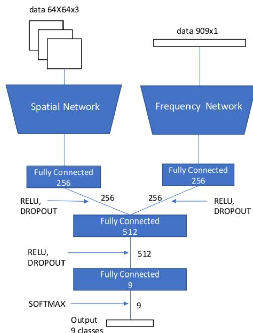
**Figure 4.** Architecture of the multi-domain convolutional neural network proposed in [65] for double JPEG compression detection.
