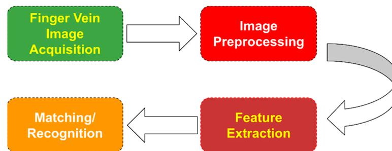
**Figure 1.** Finger vein feature extraction flowchart.
