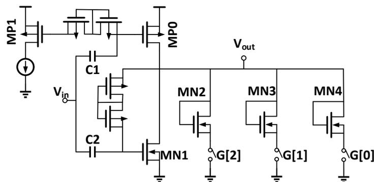
**Figure 6.** Classic neural amplifier topology with capacitive feedback.
