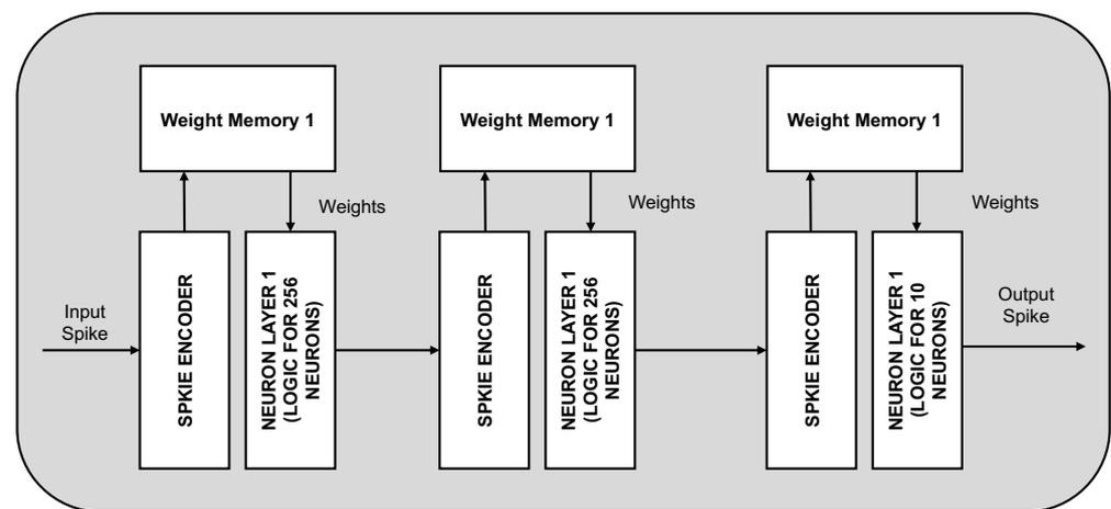
**Figure 7.** Block diagram of the neuromorphic hardware proposed by Yin et al. [49]. The architecture achieves a high level of energy efficiency by fixing the size of the network to a three-layer, 256-256-10 configurations. The input spikes for each layer are encoded by the spike encoder to select only the active neurons. Based on these indexes, corresponding weight values are fetched and loaded to the neurons calculation logic. Dedicated SRAM to store the weights of each layer is included.
