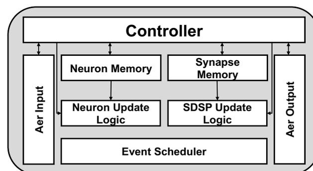
**Figure 6.** ODIN chip block-level diagram by Frenkel et al. [48]. The chip supports a form of online learning based on Spike-driven synaptic plasticity (SDSP). Local neuron memory and synapses memory is used to time-multiplex the dynamics of 256 neurons, using only a single neuron logic. The inputs and outputs of the chip use AER protocol to handle event-driven, asynchronous outputs. The neuron update logic supports both simple LIF and Izhikevich [16] neuron models.
