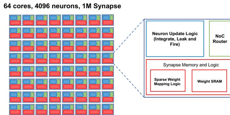
**Figure 8.** Block diagram of the neuromorphic chip proposed by Chen et al. [51]. The architecture consists of 64 neuromorphic cores, connected with a custom NoC. Each core has separate synapse memory and neuron update logic, which can support up to 64 neurons per core. High energy efficiency is achieved with a sparse connection mapping between neurons.
