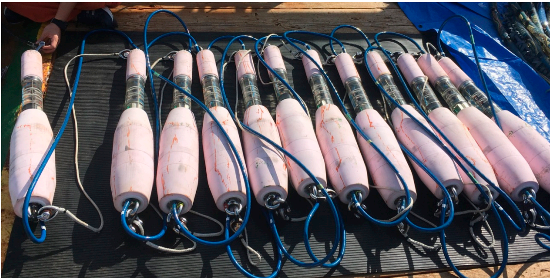
Figure 8. Photograph of 12 catenated acoustic modules with buoyancy materials being prepared for deployment on the ship.
