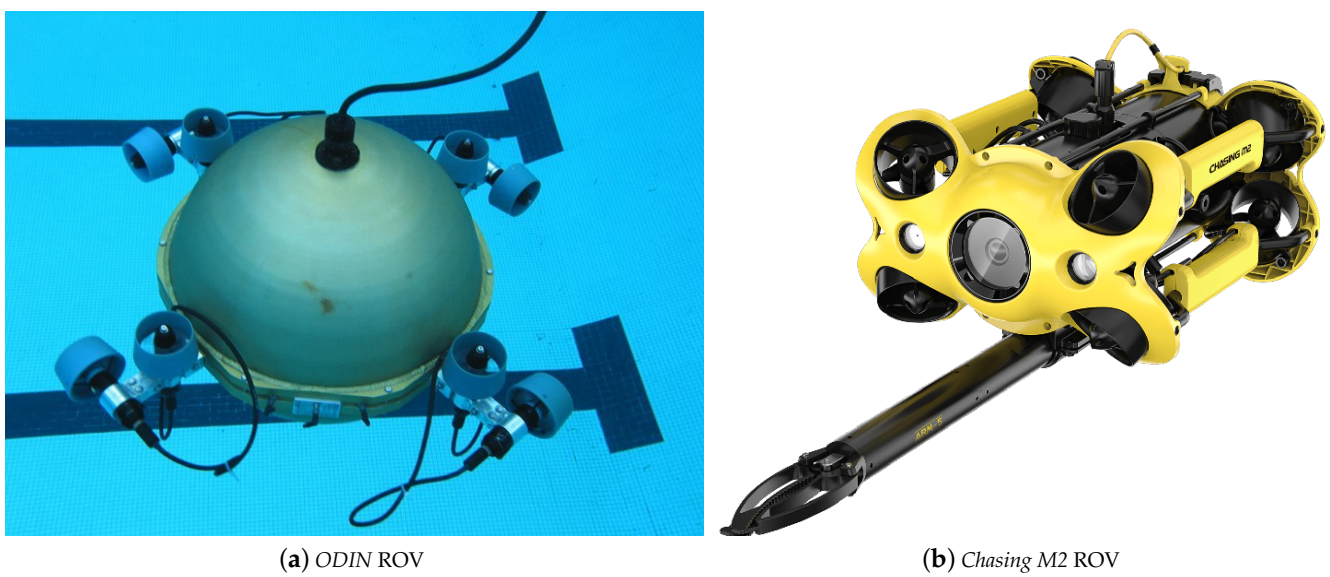
Figure 4. Examples of robots with fixed vectorial thrusters [32,42,43].
