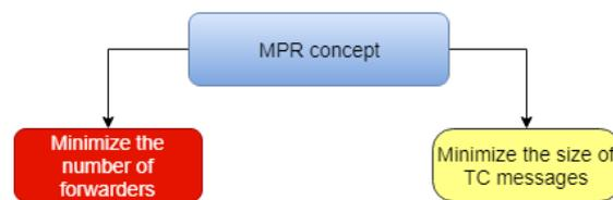
Figure 2. MPR concept of Optimized Link State Routing protocol.
