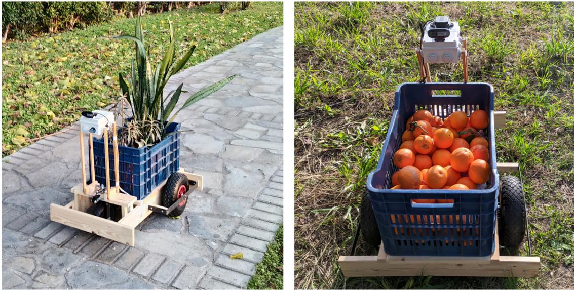
**Figure 8.** The robotic vehicle in action: the high-level controlling parts, inside the IP55 box, are clearly distinguished as well as the plastic pallet bin carrying testing cargos of 10–15 kg, approximately, on smooth (at the left) and comparatively rough (at the right) terrains.
