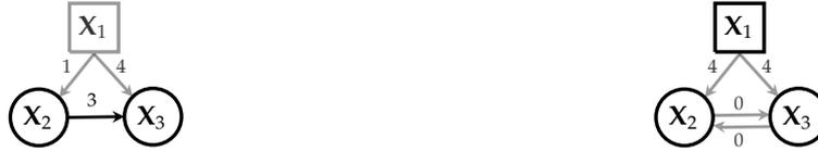
(a) TCDF will incorrectly discover a causal relationship from  $X_2$  to  $X_3$  when the delay from  $X_1$  to  $X_2$  is smaller than the delay from  $X_1$  to  $X_3$ . (b) TCDF will discover a 2-cycle between  $X_2$  and  $X_3$  where both delays equal 0, such that there should exist a hidden confounder between  $X_2$  and  $X_3$ .
