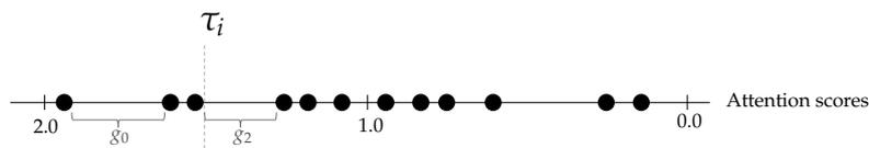
**Figure 7.** Threshold  $\tau_j$  is set equal to the attention score at the left side of the largest gap  $g_k$  where  $k \neq 0$  and  $k < |\mathbf{G}|/2$ . In this example,  $\tau_j$  is set equal to the third largest attention score.
