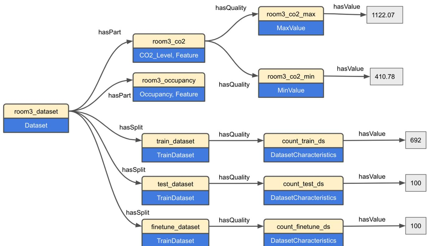
**Figure 5.** Part of the knowledge graph describing dataset features such as occupancy, CO<sub>2</sub>, and their corresponding metadata.
