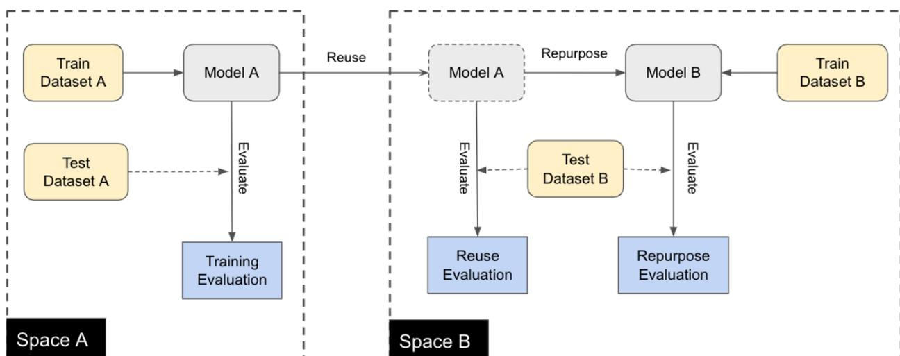
Figure 4. Methods for reusing the cognitive knowledge captured as machine learning models.
