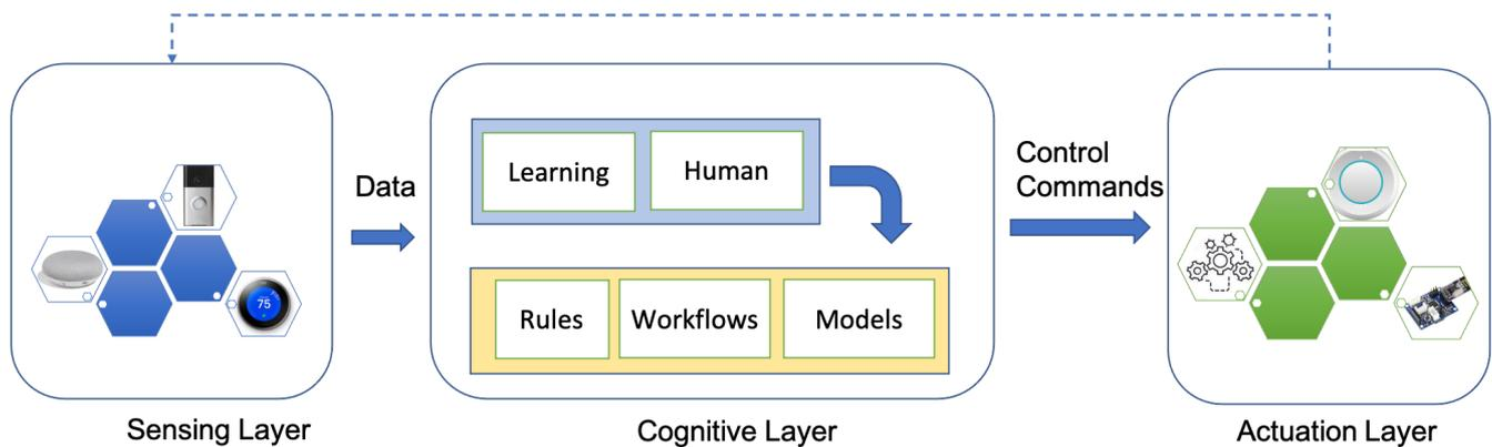
**Figure 1.** Three-layer model of an Internet of Things (IoT)-based system including sensing, context, and actuation layers.
