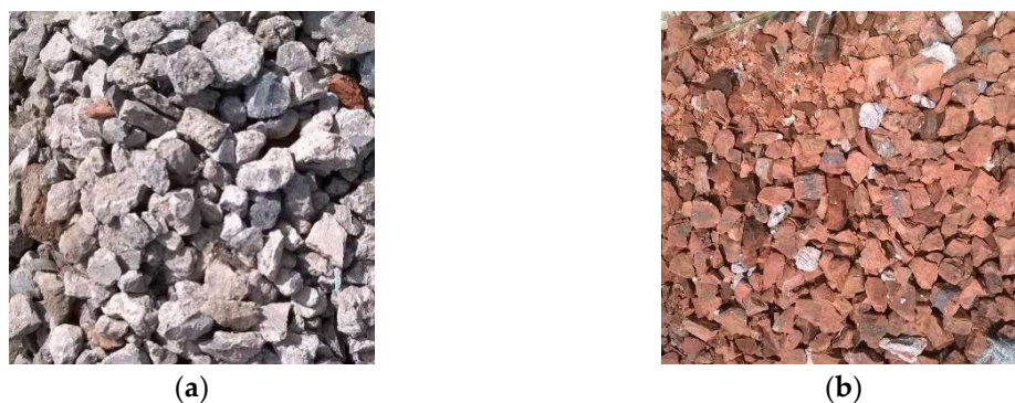
Figure 1. Recycled aggregates: (a) recycled concrete aggregate (RCA); (b) recycled brick aggregate (RBA).
