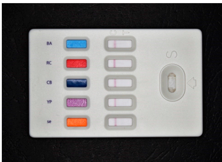
Figure 1. Example of a colorimetric, commercially available, biosensor on the principle of lateral flow assay for the determination of Bacillus anthracis (indicated by letters BA on the biosensor), ricin (indicated by letters “RC”), botulinum toxin (indicated by letters “CB”), Yersinia pestis (indicated by letters “YP”), staphylococcal enterotoxin B (indicated by letters “se”).
