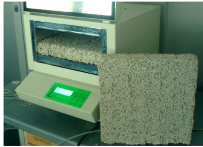
Figure 2. Heat flow meter—Fox 314 apparatus with the hemp–lime composite (Wall mix A) sample.
