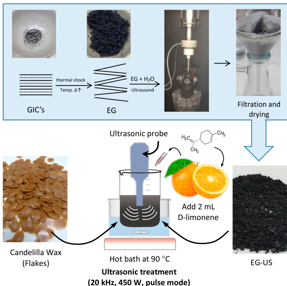
Figure 2. Scheme of the preparation of expanded graphite (EG)–wax nanocomposites. GIC, graphite intercalate compound.
