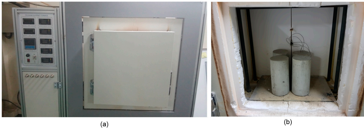
Figure 1. The electric furnace used for heating and cooling of concrete cylinders in this study: (a) a control unit and exterior view of the furnace, and (b) inside the furnace.
