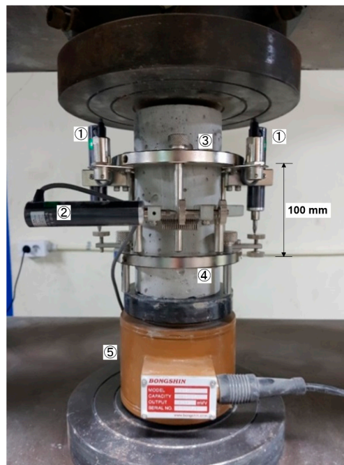
Figure 7. Test setup for the uniaxial compressive test for measurements of compressive strength, static elastic modulus and static Poisson's ratio of concrete cylinders: ① extensometers for measuring longitudinal deformation; ② an extensometer for measuring transverse deformation; ③ and ④ upper and lower fixed aluminum ring for installing extensometers, respectively; and ⑤ load cell.
