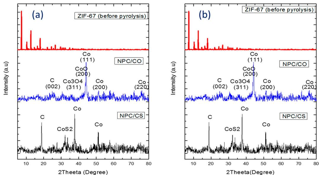
**Figure 2.** XRD patterns of (a) ZIF-67, NPC/CO and NPC/CS prepared in H<sub>2</sub>O and (b) ZIF-67, NPC/CO, and NPC/CS prepared in MeOH.
