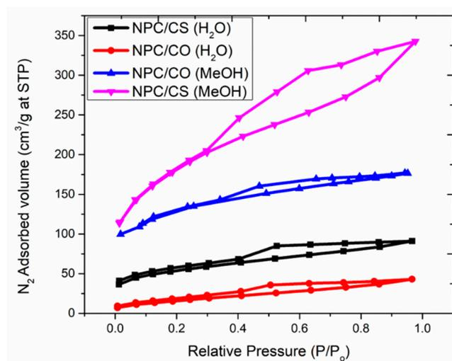
**Figure 5.** N<sub>2</sub> adsorption isotherms at 77 K.
