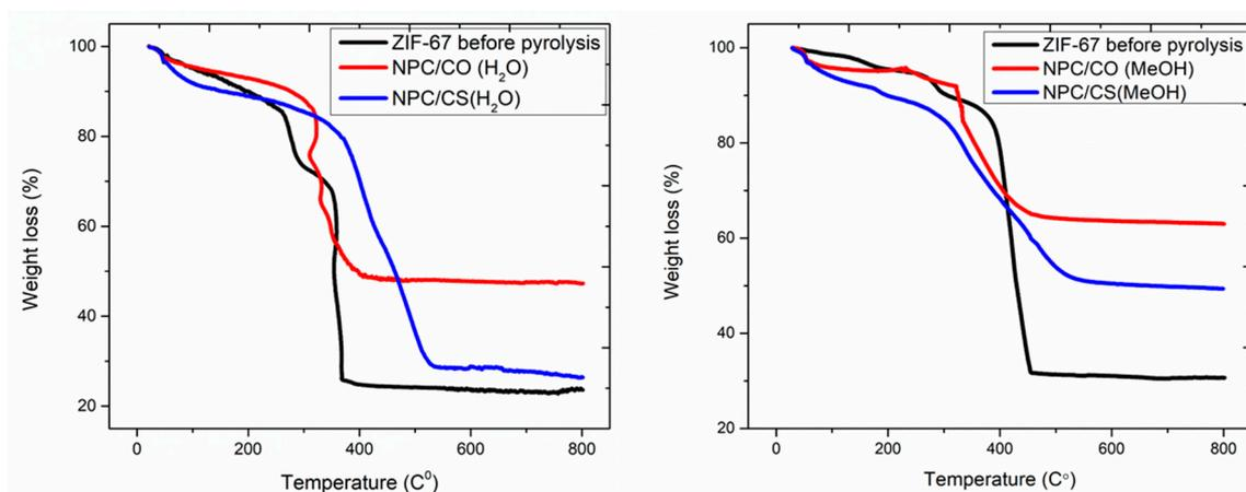
Figure 4. TGA curve analysis of as prepared ZIF-67, NPC/CO, and NPC/CS.
