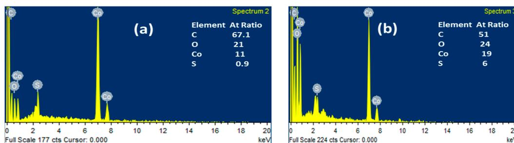
Figure 3. EDS spectrum of (a) NPC/CS (H<sub>2</sub>O) and (b) NPC/CS (MeOH).
