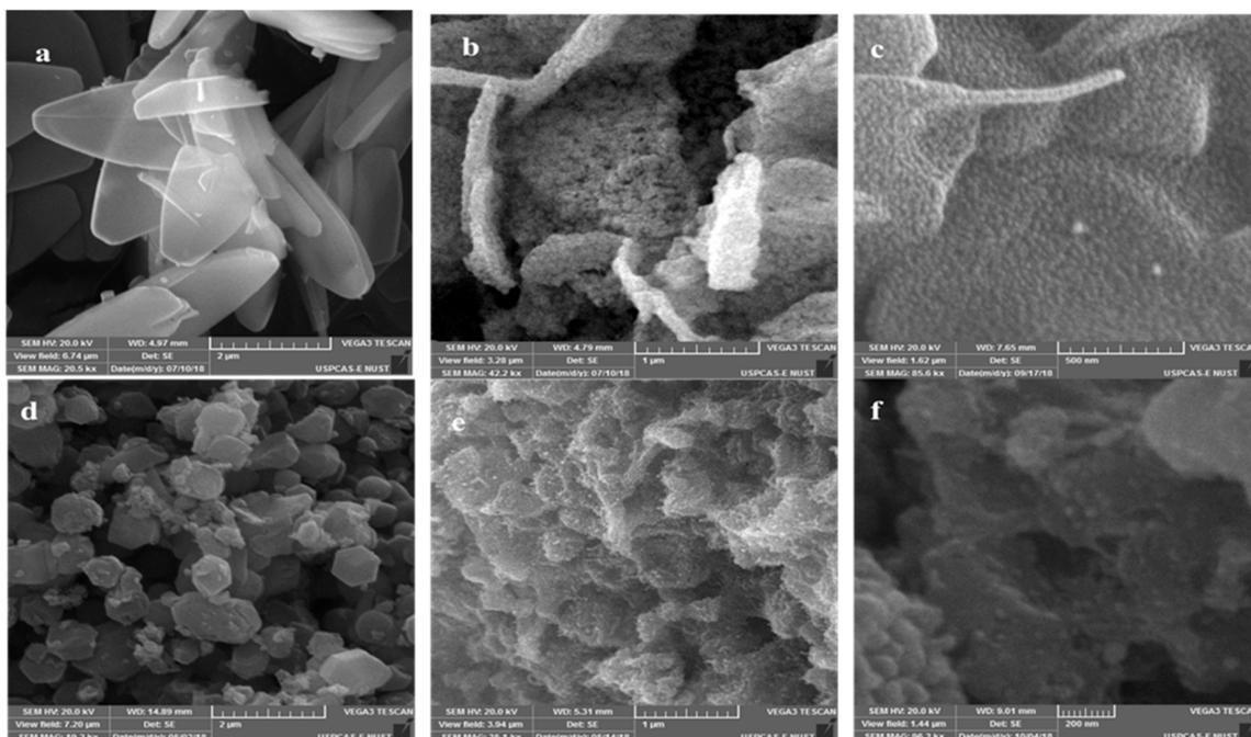
**Figure 1.** SEM images of ZIF-67 prepared in different solvents: (a) ZIF-67 prepared in H<sub>2</sub>O, before pyrolysis, after pyrolysis; (b) NPC/CO (H<sub>2</sub>O) at 700 °C; (c) NPC/CS (H<sub>2</sub>O); (d) ZIF-67 prepared in MeOH; (e) NPC/CO (MeOH) at 700 °C; and (f) NPC/CS (MeOH).
