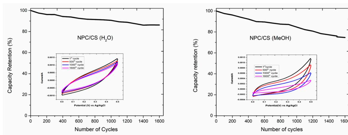
**Figure 7.** Numbers of cycles versus capacitive retention for the electrode NPC/CS electrode materials recorded over 1600 cycles at a scan rate of 100 mV/s.
