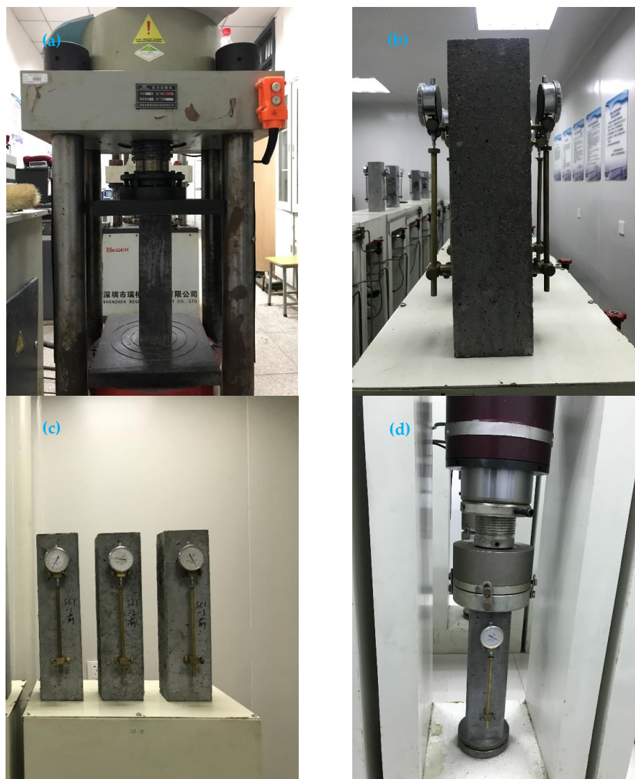
Figure 3. Experiment procedure: (a) concrete axial compression test; (b) micrometer gauge installation; (c) concrete shrinkage test; (d) concrete creep test.
