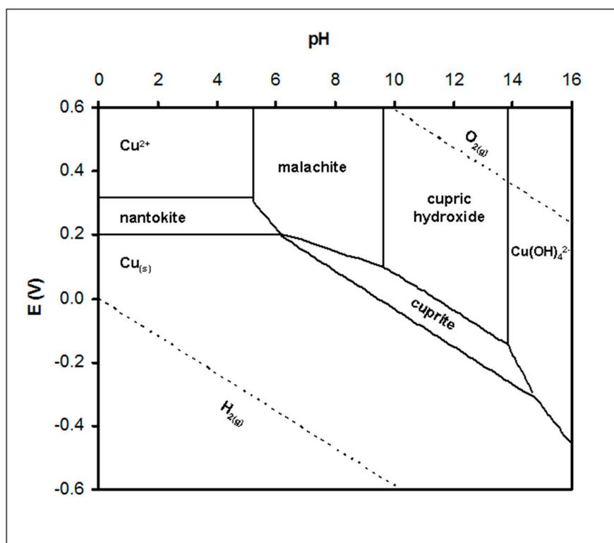
**Figure S4.** Pourbaix diagram of the corrosion by-products formed on the metallic surface of a copper-chlorine-carbonate system at 25 °C (respect to SHE). Concentrations increased  $10^3$  times in order to simulate high availability of hydrogen ion, chloride, and dissolved inorganic carbon at the metal-liquid interface.
