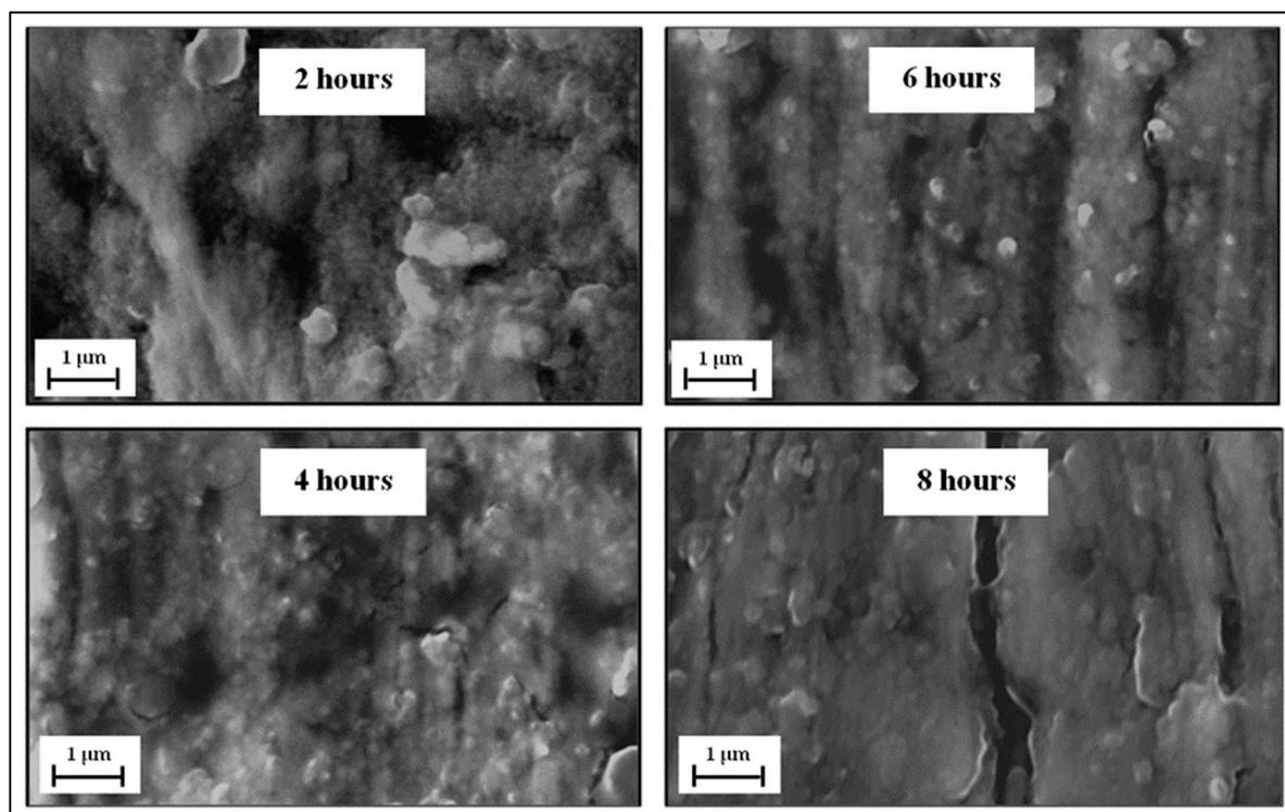
**Figure S3.** Scanning electron microscopy (SEM) images of new copper pipes in stagnant conditions with synthetic water (chlorine concentration of 4 mg/L, DIC of 80 mg as CaCO<sub>3</sub>, and pH 7.2). Images show homogeneous superficial films (identified by GI-XRD as mainly malachite).
