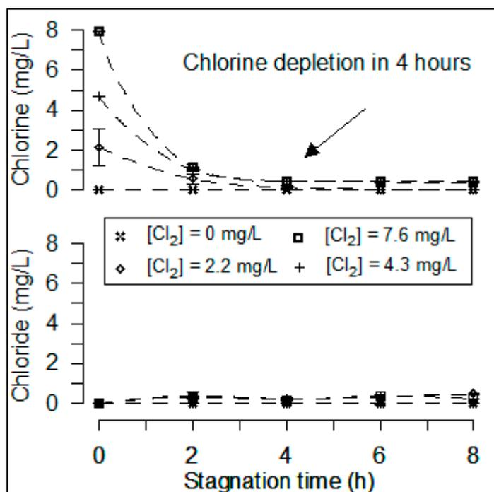
**Figure S2.** Pipe tests conducted with different initial concentrations of free chlorine. Results of chlorine consumption indicate that after approximately 4 hours, chlorine added with disinfection purposes is depleted. Measurements of chloride during stagnation suggest that most of the free chlorine is reduced to chloride precipitated during stagnation.
