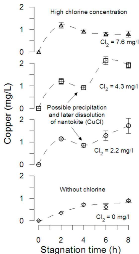
**Figure 2.** Copper release during stagnation. Pipe tests with different initial concentrations of chlorine. The error bars represent the standard deviation of the measurement ( $n = 2$ ). Initial DO was  $7.45 \pm 0.12$  mg/L.
