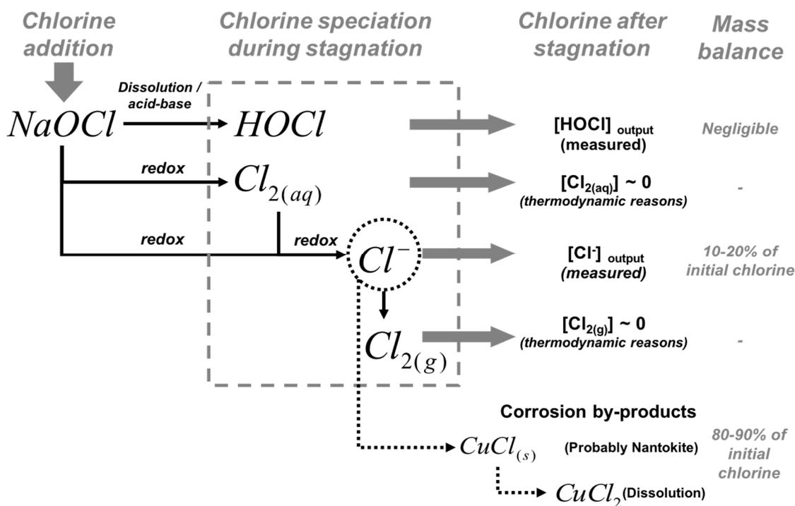
**Figure 5.** Speciation of free chlorine during stagnation. According to thermodynamic consideration and a mass balance of chlorine within the pipe during stagnation, most of the reduced chlorine precipitates as corrosion by-products, probably nantokite ( $\text{CuCl}$ ).
