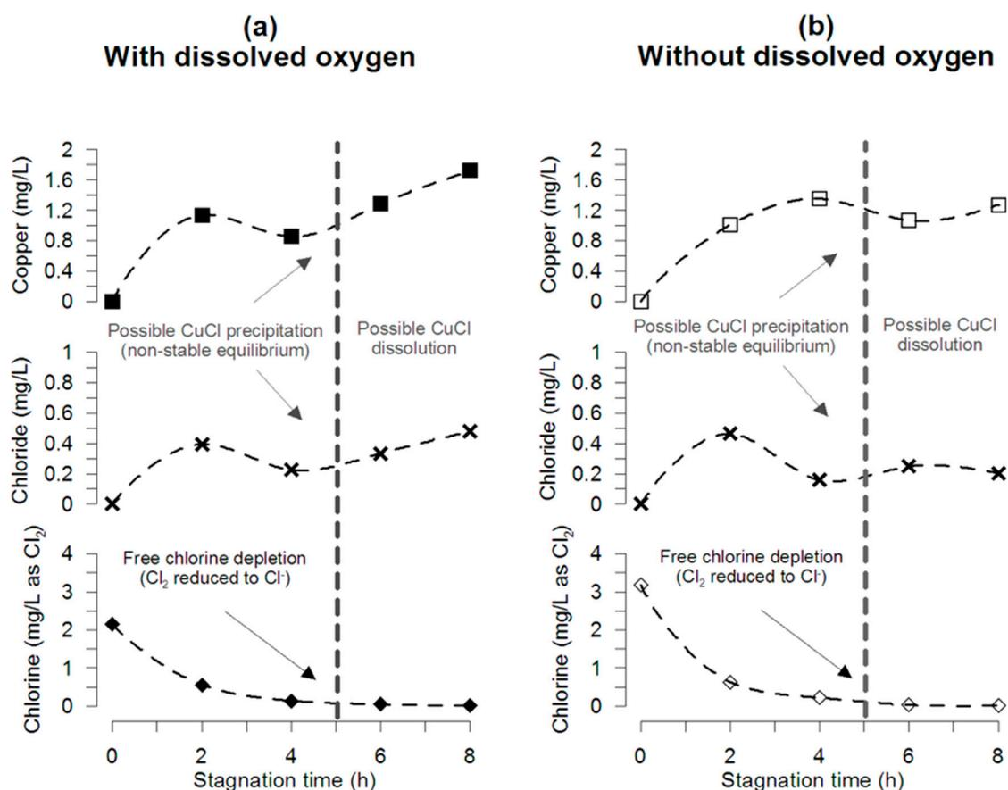
**Figure 3.** Mass balance during stagnation. A decrease in the copper concentration is reached at 4 h, probably because of Cu-Cl precipitation during the first hour of stagnation. The pipe experiments were conducted using water (a) with oxygen ( $7.59 \pm 0.00$  mg/L), and (b) without oxygen. Interestingly, in both cases, copper and chloride present a minimum concentration at the time that chlorine is almost completely depleted ( $0.02 \pm 0.00$  mg/L).
