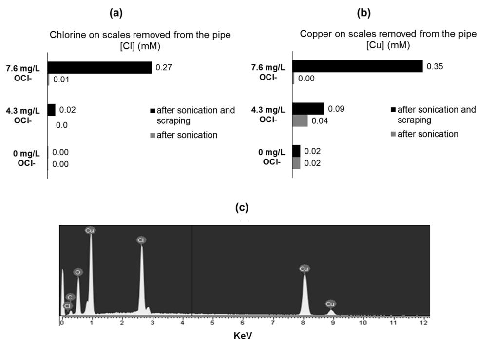
**Figure 4.** T-XRF measurements of scales removed from the tested copper pipes. Scales removal was done through simple coupon sonication and sonication-scraping (a) Chlorine, (b) Copper, (c) EDS analysis of the corrosion by-products extracted from the inner-surface of a copper stagnated for 8 hours with synthetic water (DIC = 80 mg CaCO<sub>3</sub>/L; OCl<sup>-</sup> = 8.0 mg Cl<sub>2</sub>/L).
