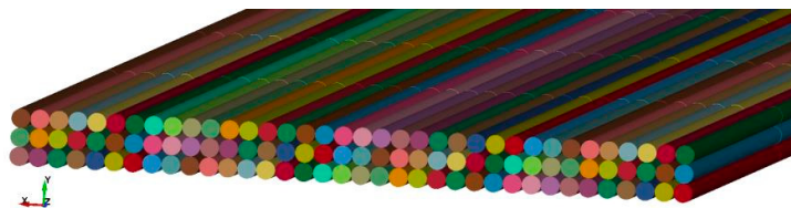
Figure 1. Micro-scale model of a multifilament fiber roving with beam element chains.
