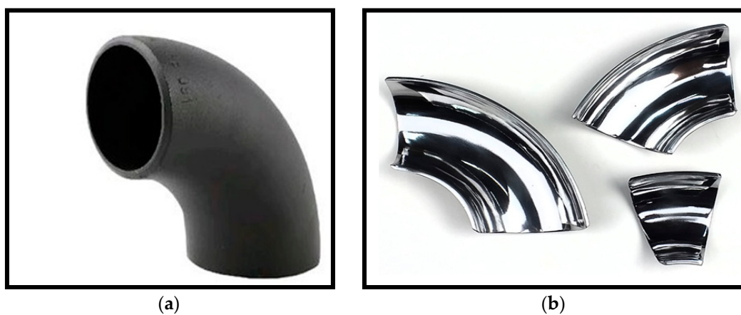
Figure 1. Carbon steel elbow specimen. (a) As received, and (b) fine polished axially cut sections.
