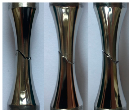
Figure 6. Fractography after the fatigue test.
