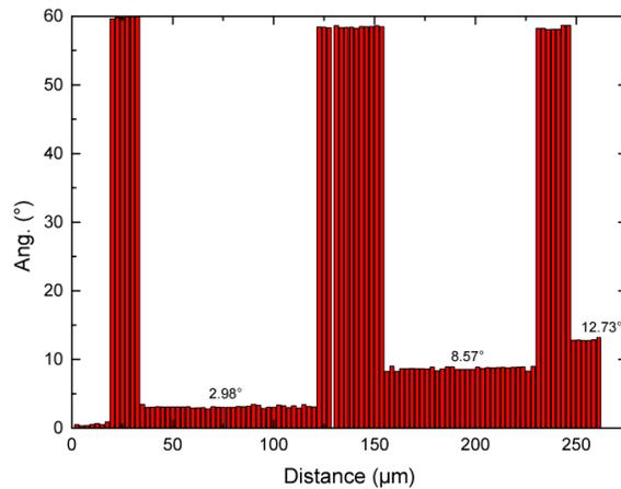
**Figure 4.** Relative misorientation angles along the red dashed-line of Figure 3, from left to right. The angle corresponds to the rotation between twinned or untwinned regions with respect to the initial region of the feathery grain.
