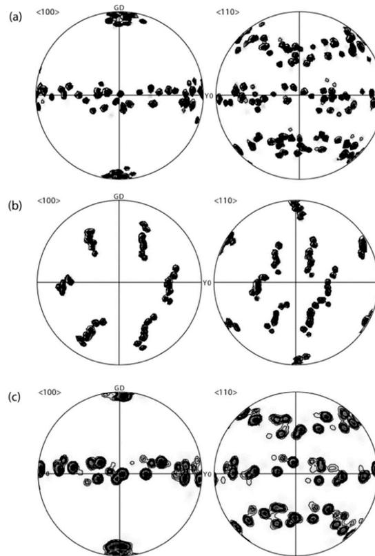
**Figure 2.**  $\langle 100 \rangle$  and  $\langle 110 \rangle$  pole figures corresponding to rectangles shown in Figure 1 with the same orientation: (a) Al-Zn sample; (b) feathery grain; and (c) “regular” columnar zone in the Al-Zn:Cr sample. The thermal gradient (or growth) direction (GD) is vertical, as indicated on the pole figures.
