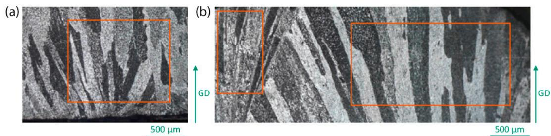
**Figure 1.** Microstructure of FFD samples: (a) for Al-20wt.%Zn alloy close to the copper chill and (b) for Al-20wt.%Zn:0.1wt.%Cr at 1.5 mm from the copper chill. The rectangles indicate the position where EBSD analysis was done.
