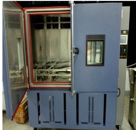
Figure 2. Programmable temperature and humidity alternating test chamber (ETE-GDJS-015L).
